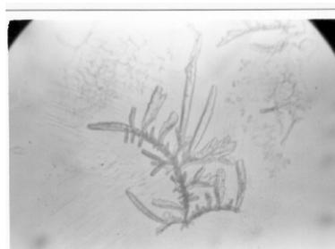
002: Dendrite Structure formed in alcoholic Phloroglucinol at  $-20.4^{\circ}$  C.
