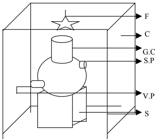
(C= Cold Room, S.P.= Seeding Port, V.P.= Vapor Port, G.C.= Glass Chamber, S= Stand, F= Fan)
